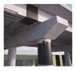
Nitowrap CWS is a 0° unidirectional carbon fibre sheet with high strength and high elastic modulus. It is used with specially developed resins 'Nitowrap 30 Primer' and 'Nitowrap 410 saturant' and externally applied to concrete or masonry. When correctly designed and applied, the Nitowrap system may improve structural load carrying capacity, flexural strength, shear strength and provide resistance to deformation.
